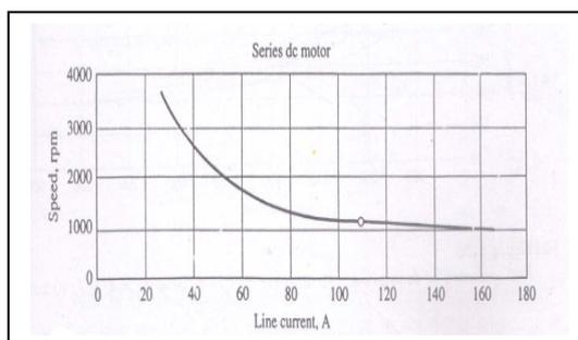
Fig.2.c.Series DC Motor Of Starting Current Characteristic
