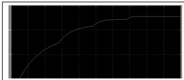
Fig.5a. The Result of Starting Speed dc motor with Variable Regenerative Control
