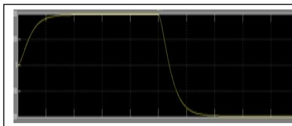
Fig.5b. The Result of Starting Speed dc motor with BJT-H Bridge Control
