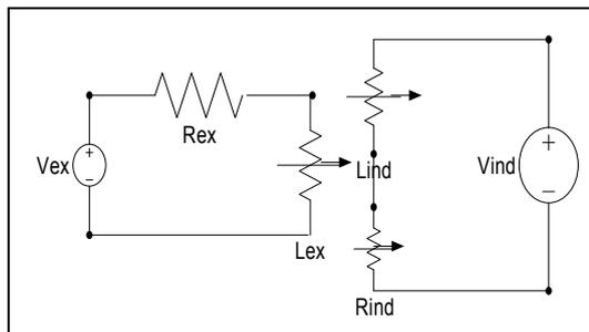
Fig.2.a. Series DC Motor equivalent circuit Model
