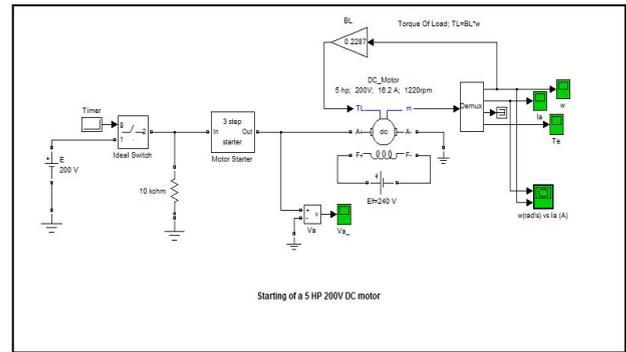
Fig. 1a. DC Motor With Variable Control Circuits Model
