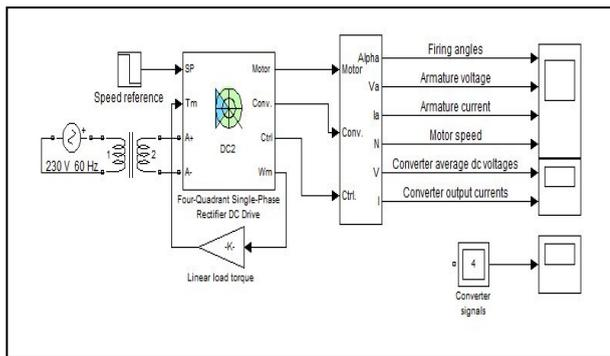
Fig.1e. DC Motor With Rectifier Control Circuits Model
