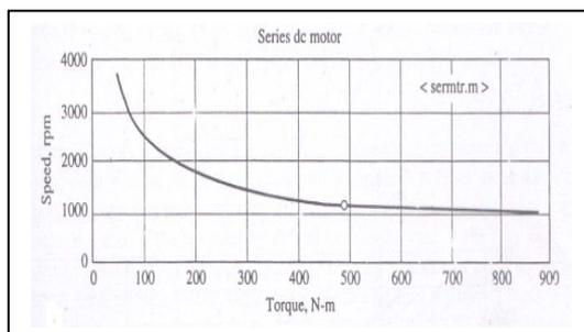
Fig.2.b.Series DC Motor Of Starting Torque Characteristic
