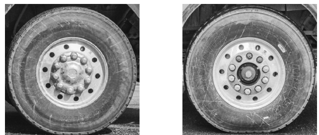
Fig. 11. Concrete truck tire Bridgestone M860A—empty vs. fully-loaded.
