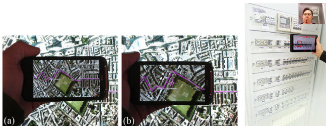
Fig. 2. (a) The dual-view problem caused by device- perspective magic-lens rendering. (b) User-perspective magic- lens rendering where such dual-view problem is not present. [71] (c) the users views AR instructions through the tablet [72].
