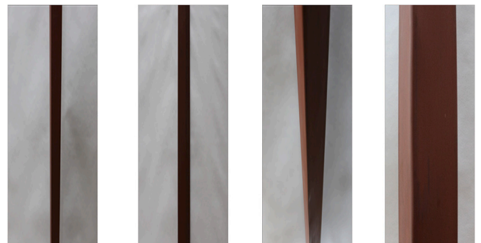
Fig. 6. Undamaged steel frame images.
