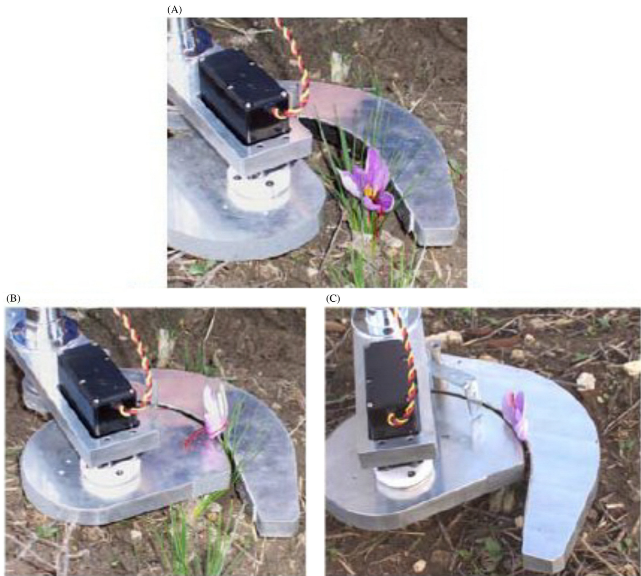
FIGURE 11.13 The field operation of the cam-strike harvesting machine: (A) approaching, (B) gripping, and (C) detaching. From Gambella, F., Paschino, F., Manuello Bertetto, A., 2013. Perspectives in the mechanization of saffron (Crocus Sativus L.) . Int. J. Mech. Control 14 (2), 3–8.
