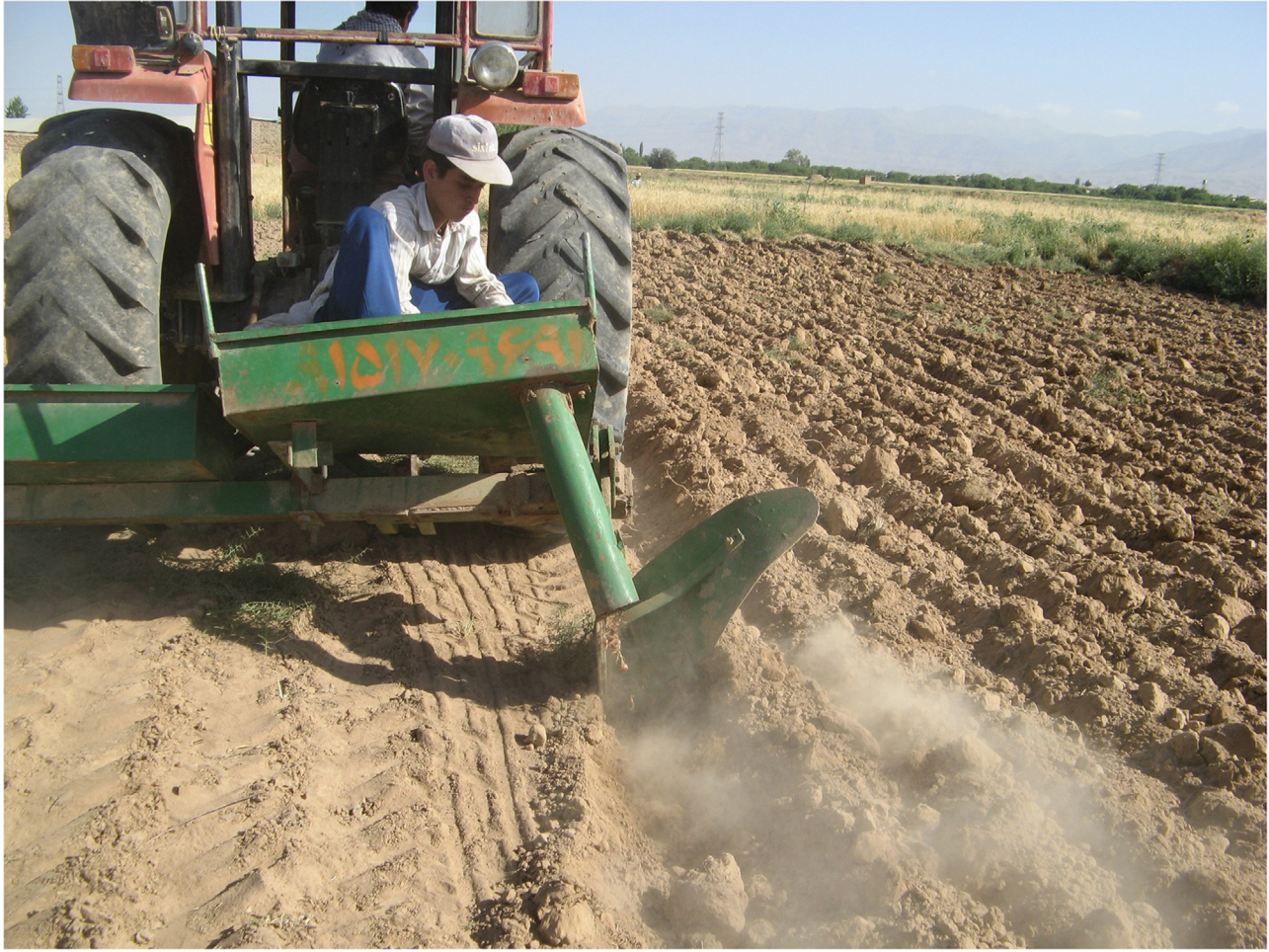
FIGURE 11.5 Single-bottom moldboard plow equipped with corm hopper. From Saeidirad, M.H., Zarifneshat, S., Mahdinia, A., Nazarzadeh, S., Mazhari, M., Mostafavand, H., et al., 2014. Investigation on mechanization development possibility and providing the most optimum method to saffron harvesting mechanization. Final Research Report, No. 44678, Agricultural Engineering Research Institute (in Persian).
