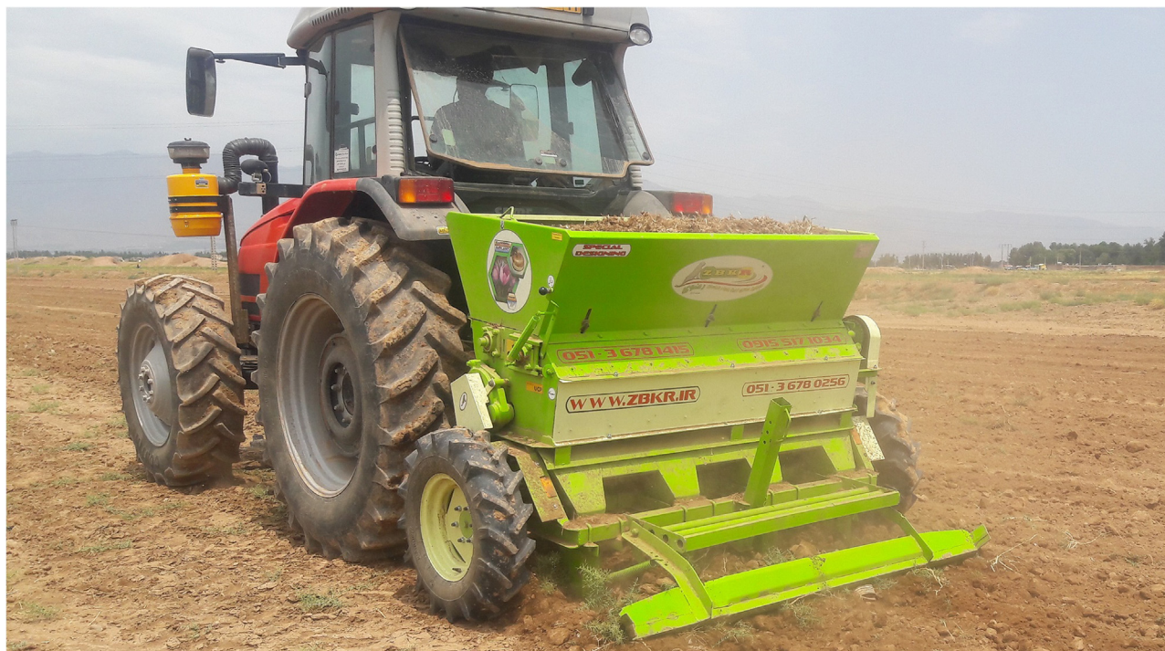
FIGURE 11.8 Fully automated seven-row saffron corm planter. From Saeidirad, M.H., Zarifneshat, S., Nazarzadeh, S., Mehrabi, E., 2018. Design, development and evaluation of 7 rows saffron corm planter. Final Research Report, No. 53999, Agricultural Engineering Research Institute (in Persian).
