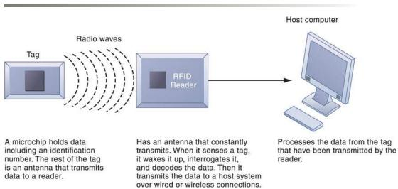
RFID uses low-powered radio transmitters to read data stored in a tag at distances ranging from 1 inch to 100 feet. The reader captures the data from the tag and sends them over a network to a host computer for processing.
