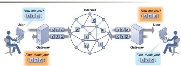
FIGURE 7-11 HOW VOICE OVER IP WORKS
