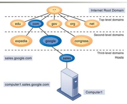
Domain Name System is a hierarchical system with a root domain, top-level domains, second-level domains, and host computers at the third level.
