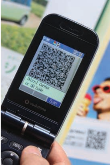
Figure 7.8 QR codes linked to specific goods and services are used by mobile phone users to retrieve product information. (Source: © jeremy suttonhibbert/Alamy)
